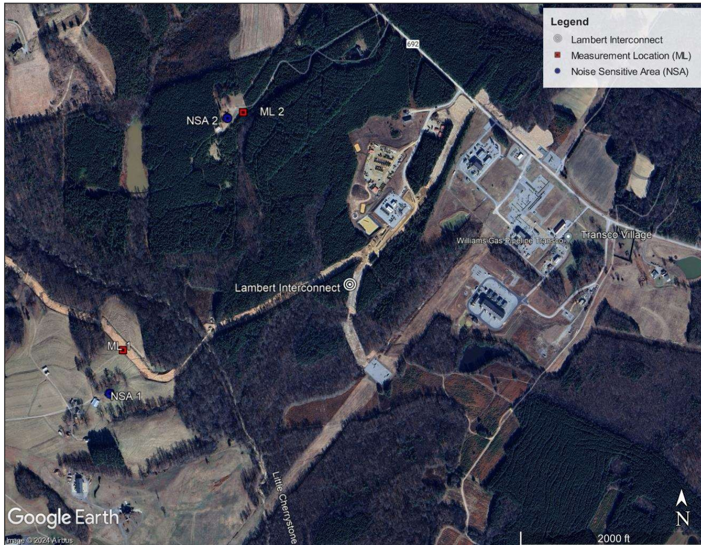
Figure 1: Lambert Interconnect NSAs and Measurement Locations
