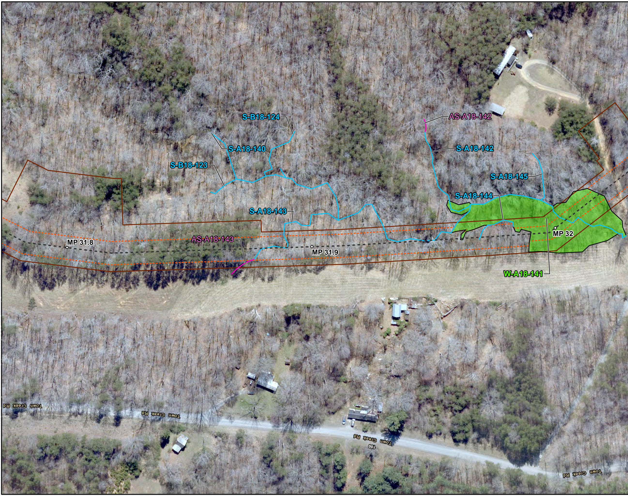
Figure 2.3-8 Construction Workspace Parallels Waterbody (or Wetland) Within 15 Feet Rockingham County, NC Sheet 4 of 18
